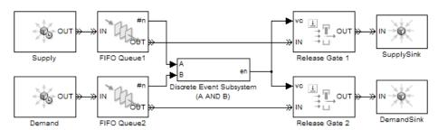
Suppose that the top queue contains one entity and an entity arrives at the previously empty bottom queue. Assuming that no block in the model has its **Resolve** simultaneous signal updates according to event priority parameter selected, the entity arrival has the following cascade of consequences:
